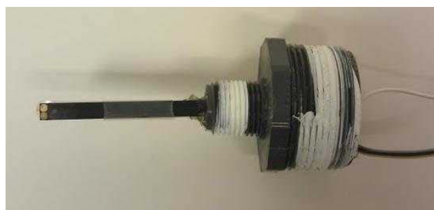
Fig.1. Photograph of waterproof package for the ISFET pH probe depicting the PVC and silicone barrier between the sensor probe and electronic connections.
