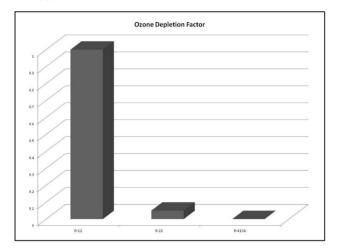
B. R-424A (RS-44): - After the ban of refrigerants like R-22, the requirement of new refrigerant was replaced by introduction of new refrigerant of future which is R-424A.
