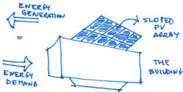
Fig.4. Conceptual sketch for a minimal formal result for the relationship between PV and the building in a one-storey building, when optimizing the PV yield.
