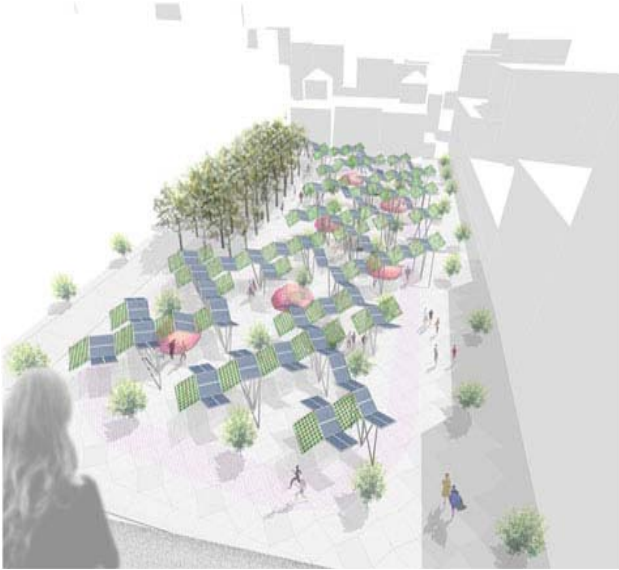
Fig. 9. Plaza del General Vara del Rey project, Madrid (Spain), 2009. PV is shaped as a pergola made of technological trees that characterize the square. Design: ELII Oficina de Arquitectura. Picture by courtesy of the architects
