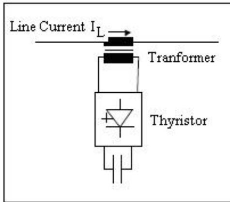
Fig. 4: Static Synchronous Series Compensator , SSSC
