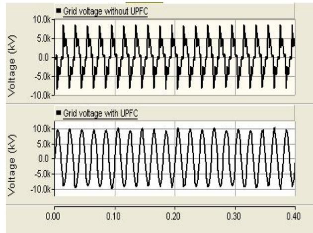
**Fig 11:** Grid voltage without UPFC and with UPFC
