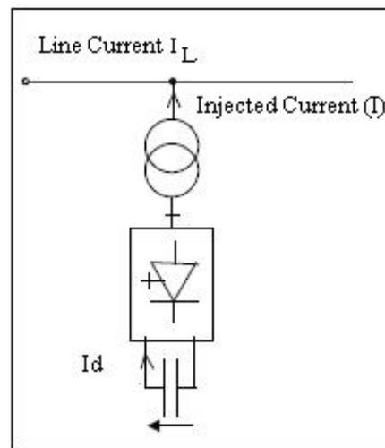
Fig. 3 : Static Synchronous Compensator (STATCOM)
