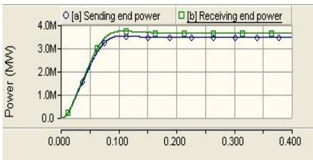
**Fig. 8 :** Sending end and receiving end active power with UPFC
