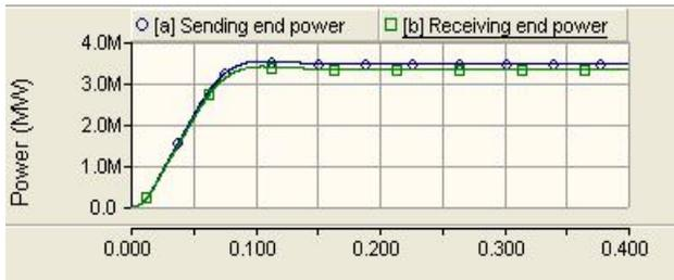
**Fig. 7 :** Sending end and receiving end active power without UPFC
