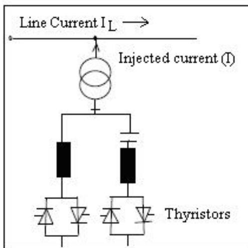
Fig. 2: Static Var Compensator (SVC)
