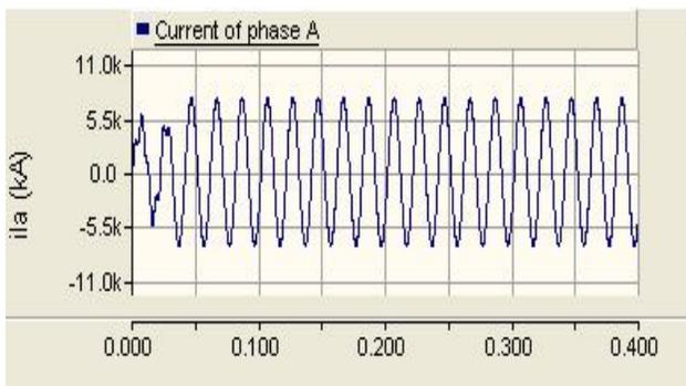
**Fig 10 :** Current of phase 'A' with UPFC
