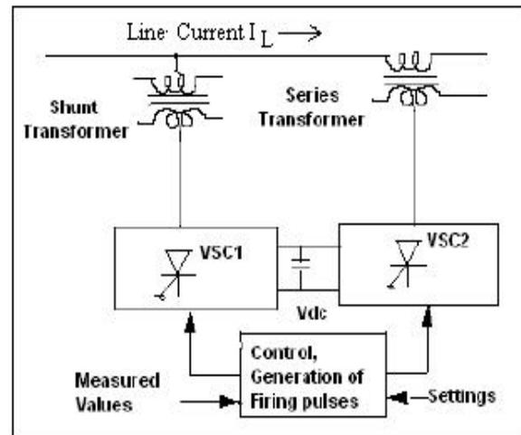
Fig. 6: Unified Power Flow Controller (UPFC)
