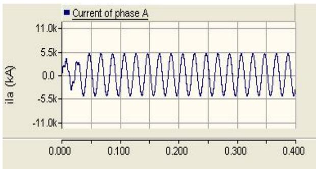
**Fig 9 :** Current of phase 'A' without UPFC
