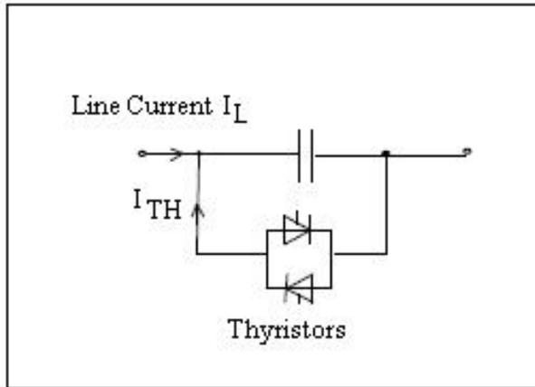
Fig. 1: Thyristor Controlled Series Capacitors (TCSC)
