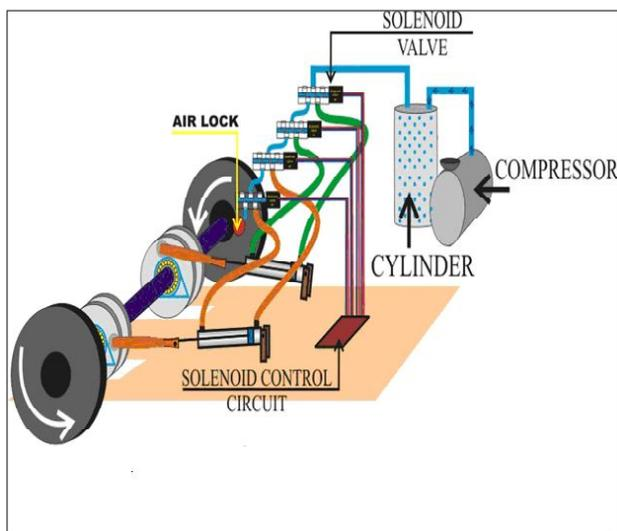
Fig. 1 : Schematic diagram of Air Engine
