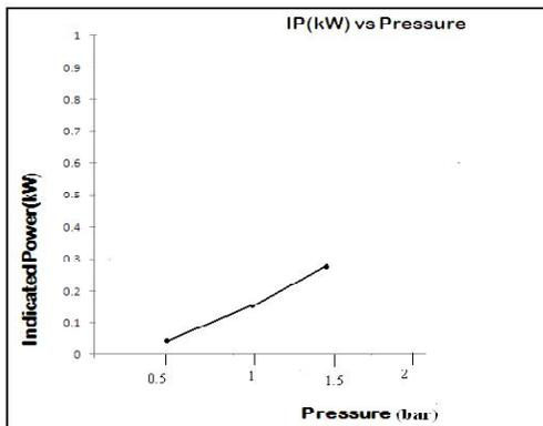
Fig. 3 : Indicated power vs pressure
