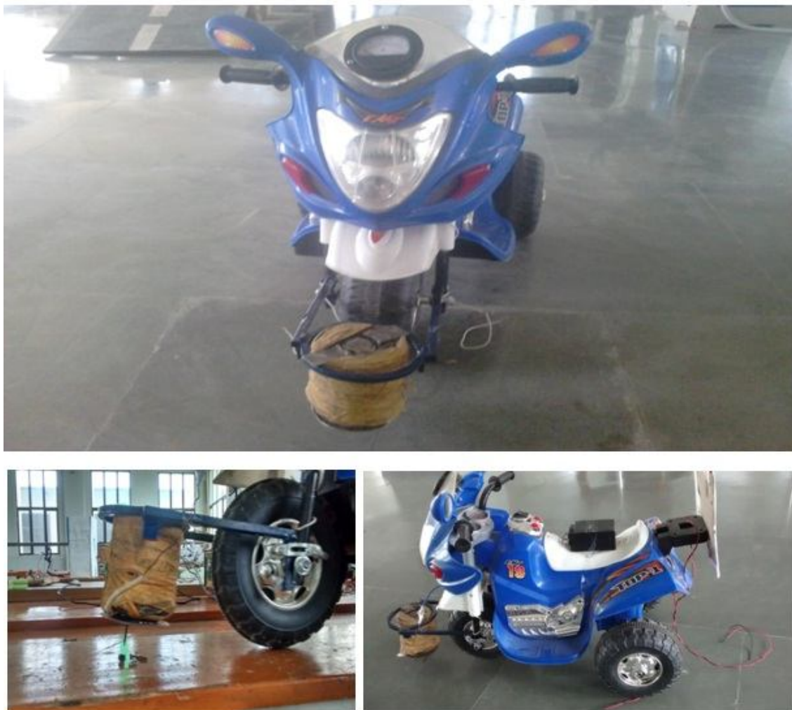
Fig.3. Workings Model of Electromagnet to Save the Tyres from Nails.
