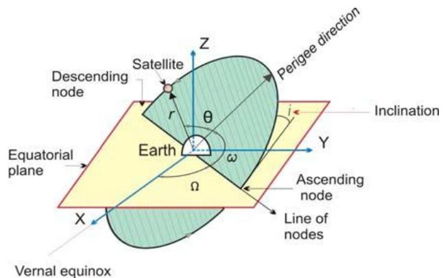
Fig. 6. Space Orbital Parameters
