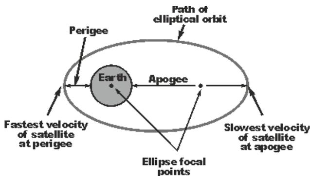
Fig. 4. Highly Elliptical Satellite Orbit, HEO
