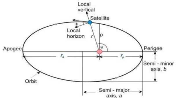
Fig. 5. Major Parameters of an Elliptical Orbit
