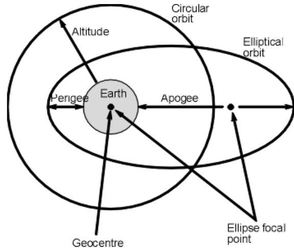
Fig. 3. Circular vs Elliptical Orbit
