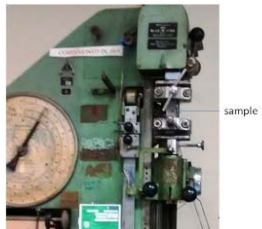
Fig.4: Testing of welded sample on UTM
