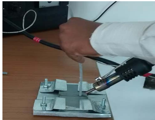
Fig.2: Hot air welding operation performing in Lab
