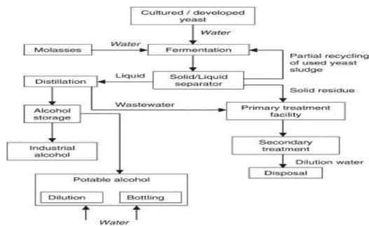
**Fig.1:** Schematic of Alcohol Manufacturing Process
